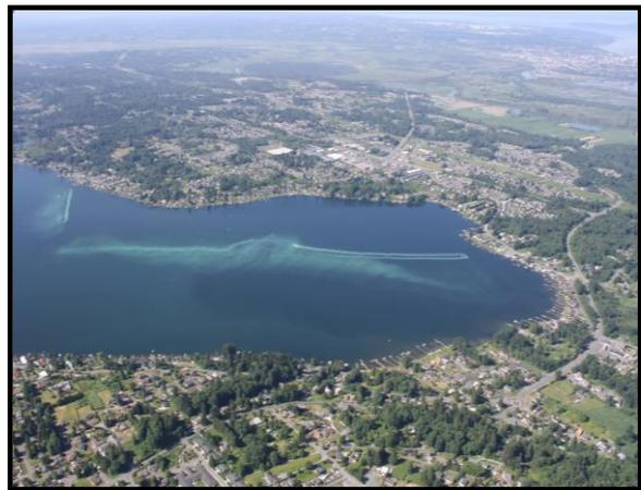
The team was faced with moving and applying 55,000 gallons of alum to the lake within a short time frame to minimize impact on lake users. Two 30 foot converted Bayliners designed to hold 500 gallon tanks were deployed to the lake, these boats were equipped with precision application guidance systems. They were able to move to the application track, apply their load rapidly, and return for the next load at 30 miles per hour, something that's important for turn around.
